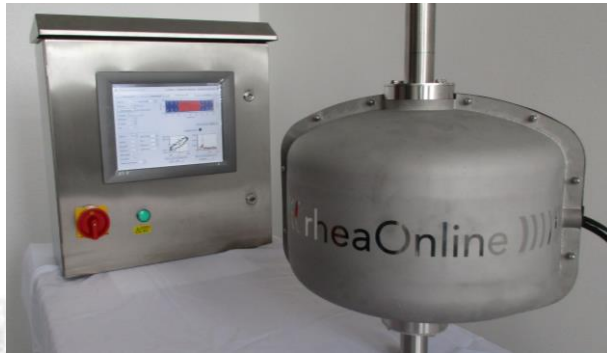
RheaOnLine, prototype 1.0, outfits agro-food and cosmetic production line pipes.
